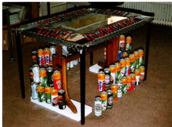
BELOW: Jig for stretching Mylar membrane
